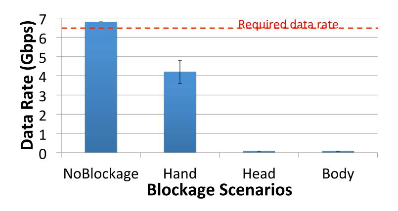
Blocking millimeter wave signals results in a significant drop in data rate
