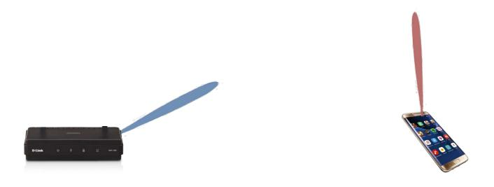
Communication is possible only when the beams are aligned
