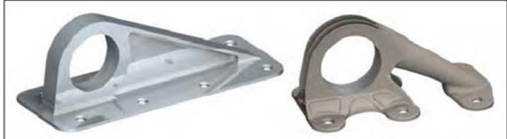
Conventionally machined bracket (left) and redesigned bracket (right) using topology optimization, courtesy of Laser Zentrum Nord GmbH and Airbus
