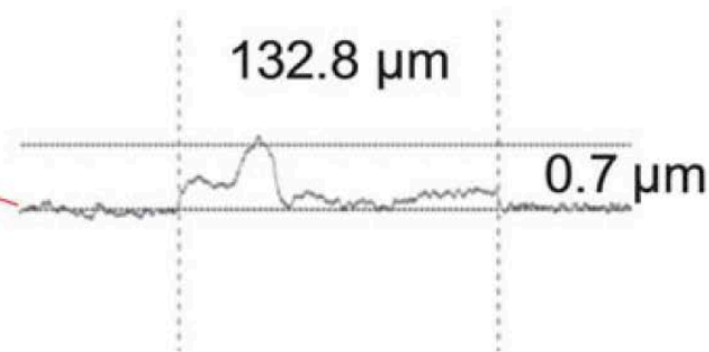
Flexographic (bottom) printed Ag NP ink [Yu et al., Nanoscale 2012]
